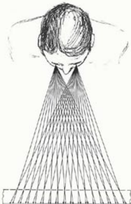
Figure 3. Sight lines through a Parallax Barrier Screen. (Roberts)
